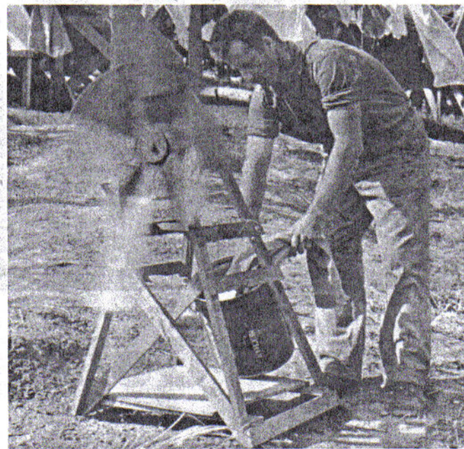
Wind power works this washing machine. Blades were made from oil drum top, plunger from howitzer shell. Wind drives plunger, agitating clothes
