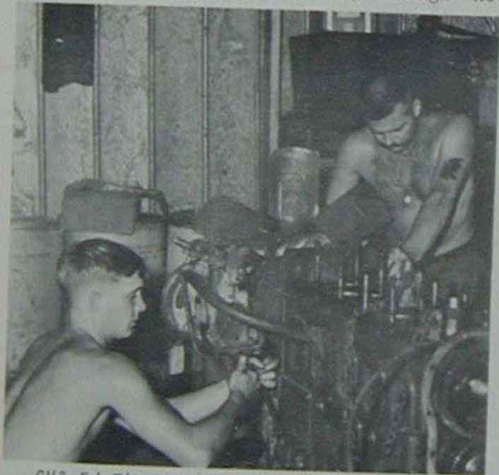
CM3 Ed Thompson (left) from Frankfurt, Kentucky and CM2 Earnest Callahan from New Castle, Pennsylvania, work on a 671 GMC Diesel Engine from a 20-ton rock dump truck.
