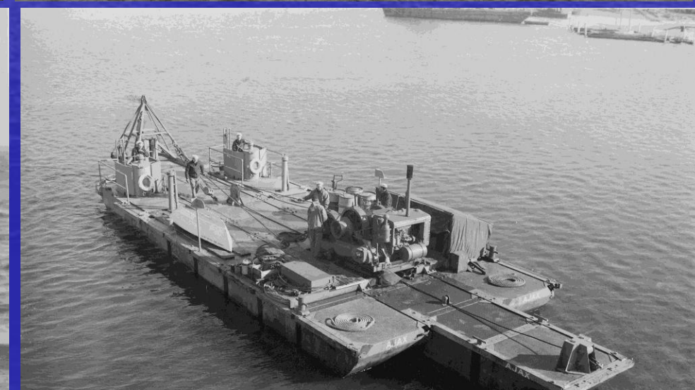
Standard pontoon warping barge, used to assemble larger pontoon barge assemblies
