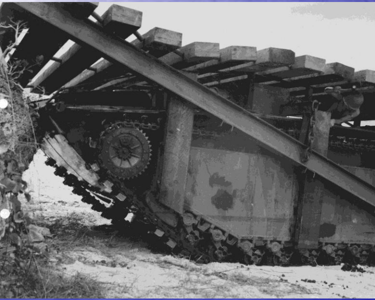
The ramps were fashioned from two 10-inch steel I-beams 25 ft long, welded to form a rectangular frame to support a flexible timber ramp
