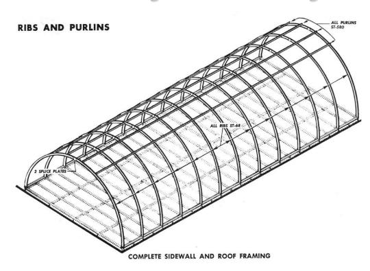
The original Quonset Huts utilized arched ribs using steel T-sections,  $2 \times 2 \times \frac{1}{4}$  inches, and the hut was only 16 by 36 ft. These were replaced by Stran-Steel's novel ribs, which were  $2 \times 3-5/8$  inches, formed by sandwiching two lightweight channels welded back-to-back (see detail in following slide)
